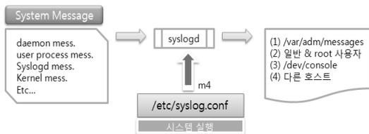
Fig. 11. principles of syslog
